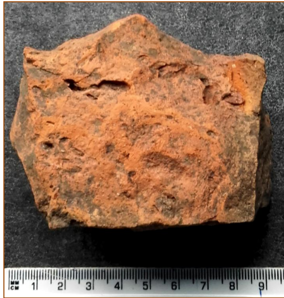
Hard red-orange ceramic building material (CBM) The ceramic is unusually consistent in colour and fabric - unlike brick Three pieces found fit together and appear to be a thick tile.
